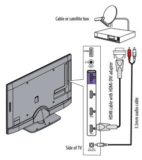
5 Connect a 3.5mm audio cable (not provided) to the PC/DVI AUDIO IN jack on the side of your TV and to the AUDIO OUT jacks on the cable or satellite box.
